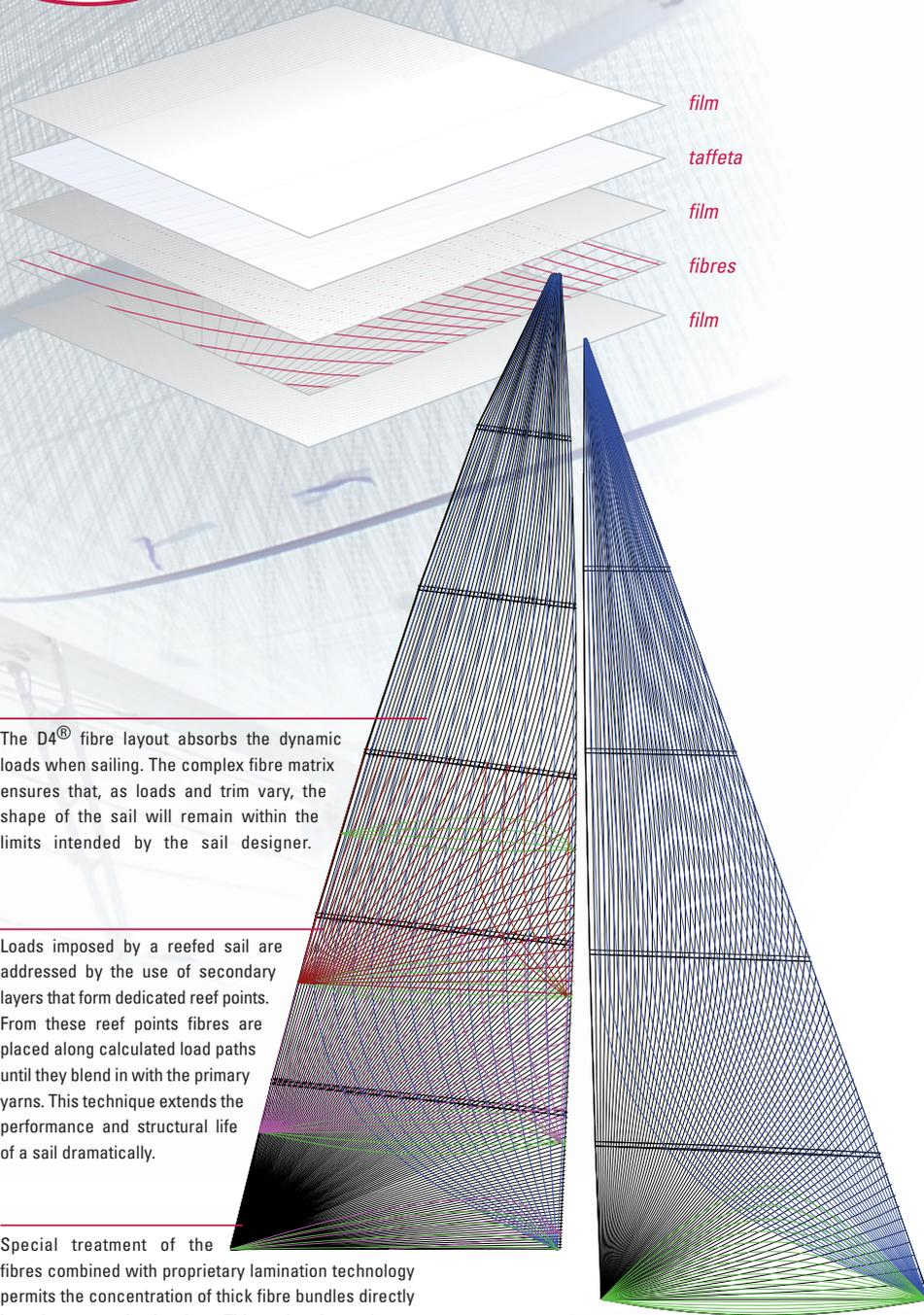
The D4<sup>®</sup> fibre layout absorbs the dynamic loads when sailing. The complex fibre matrix ensures that, as loads and trim vary, the shape of the sail will remain within the limits intended by the sail designer.
